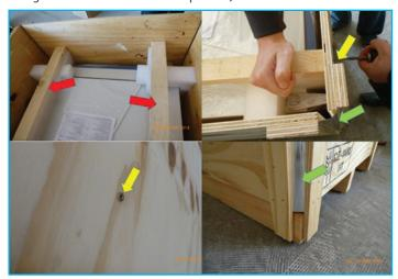
After removal of balks (if any) and all the screws it is possible to move the outer walls upside in case of small devices. In case of large devices, the package is dismantled to individual side walls that are removed. The device is moved from the palette in the same way as before.
