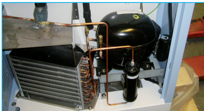
In case of CLC 404, the compressor remains to be placed in current carrier
